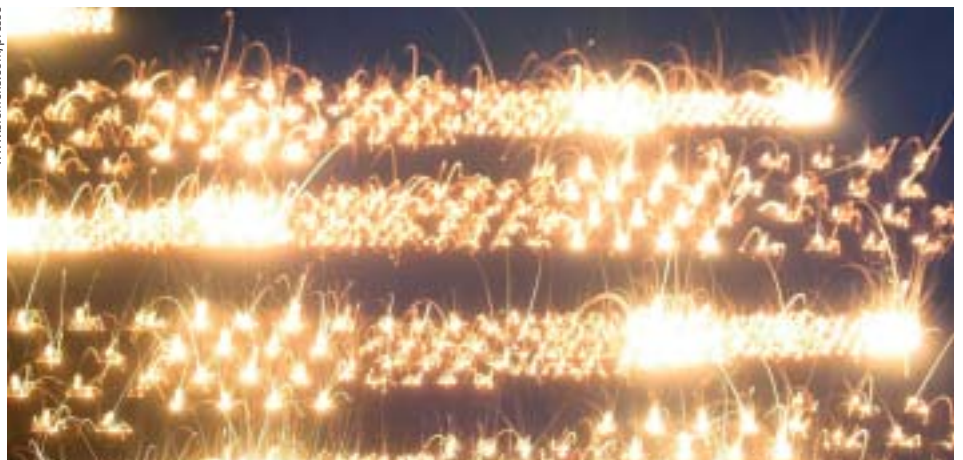
Machine parts are now being 'printed' out of metal with the help of lasers: the laser welds the metal powder to a new component in a sea of sparks, controlled by computer.
