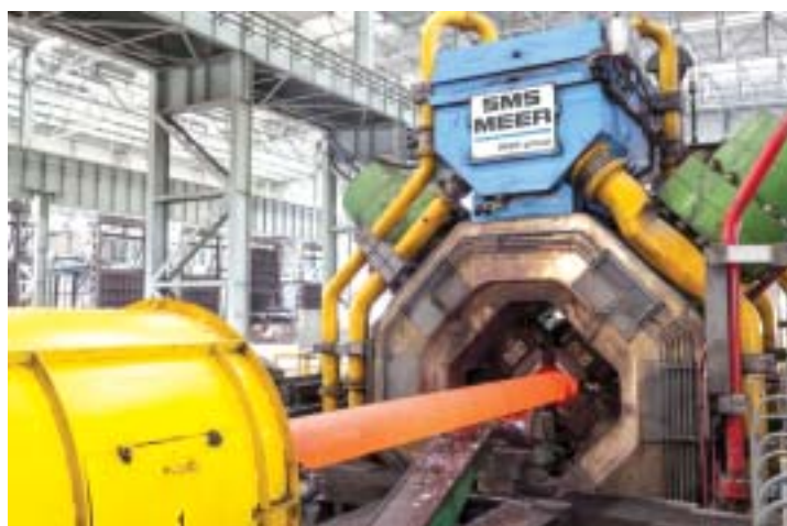
Rods with different cross sections and in different grades are being manufactured at Dongbei Special Steel in Dalian/China on a radial forging machine supplied by SMS Meer.
