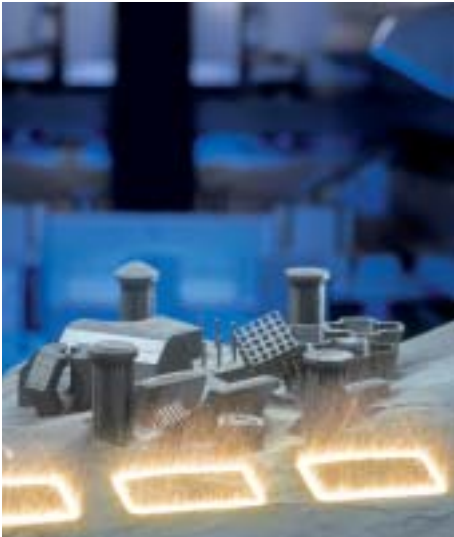
The laser beam welds the metal powder into three-dimensional structures step by step.
