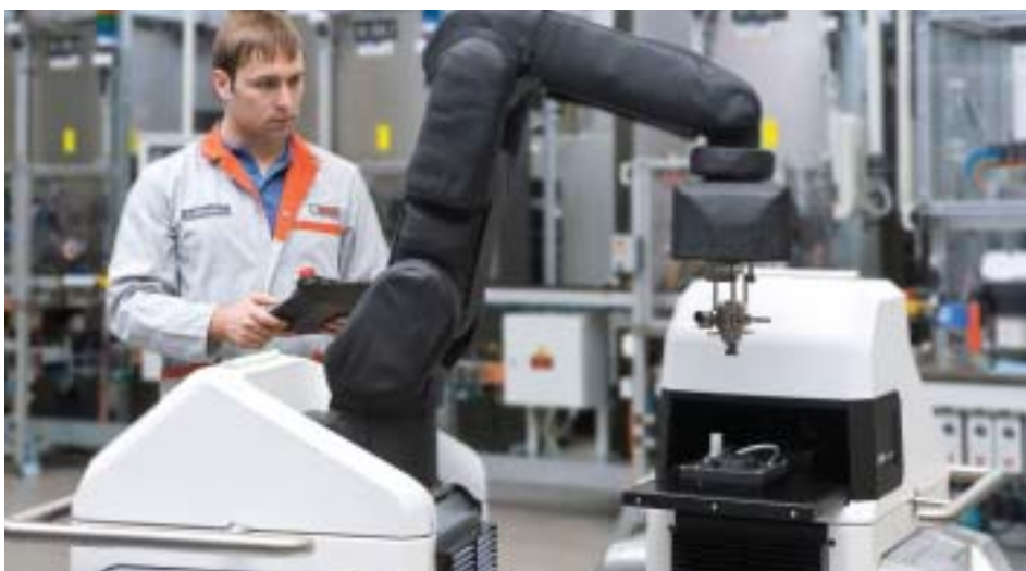
The Bosch APAS family of systems, including the APAS assistant (left) and the APAS inspector (right), are operation-ready automation solutions for industrial and other applications. Operated via a touchpad and graphical user interface, devices in the APAS family can easily be trained to carry out a variety of tasks.
