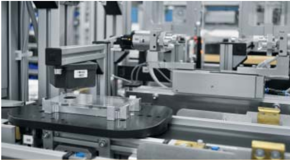
An RFID reader head records order data on a blank workpiece with wireless data carrier and initiates the next processing step accordingly.
